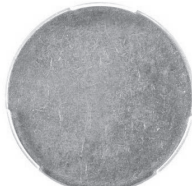
25c, 1965-22, T-2 obv-clad layer missing, 4.78g
