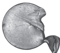
1c, T-2 Pl, rag clip torn by upsetting mill
