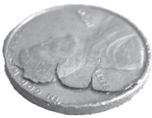
1c, cu, 1972-D, Lg Peeling Lam
