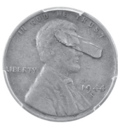
1c, cu, 1944-S, Retained Lam Peel.
