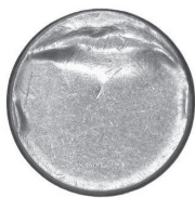
10.1, T2 clad, included gas bubble
