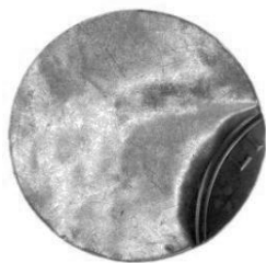
25c, ND Separated clad layer “LI”
