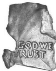
25c, ND Separated clad layer fragment
